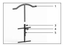
1. Insert Cross-Bow [1] handle into Cross-Bow (receptacles) frame [5]. Ensure the pop-up pin [4] and stud knob [3] are loosened (unscrewed) before attempting to pull out.
