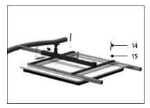
**5.** Attach Cross-Bow with the new bolts and washers [14, 15] provided. Tighten using the adjustable or 7/16" open wrench. Confirm all hex bolts [14] are tightly secured and check regularly as instructed in the "Mechanical Safety Check".
