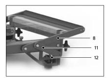
**1.** Lower the footbar [8] by adjusting the swing arm [11] of the Reformer to cradle position #4 [12].
