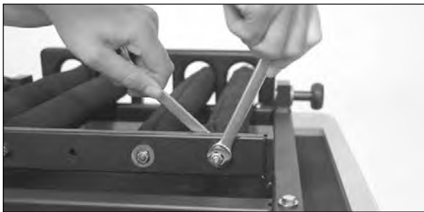
3. Using second 7/16" wrench on opposite side of spring anchoring bar, loosen nylon locknut. This may require exerting a bit of torque.
