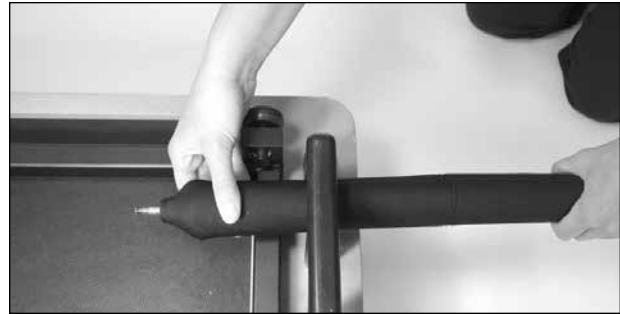
2. Insert the spring through the spring holder.
