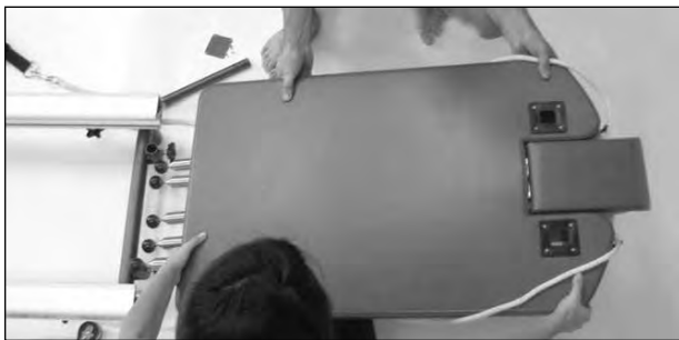
1. Remove carriage. Find full instructions on page 22 of your Reformer's Manual or view video online at merrithew.com/support/equipment-manuals-assembly
