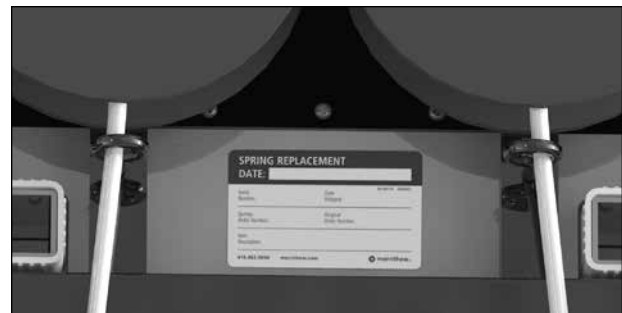
6. Affix the sticker provided with your spring replacement package to the underside of the Carriage.
