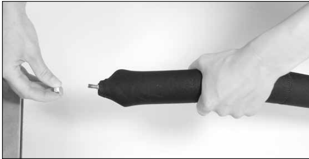
1. Remove nylon locknut from spring bolt.
