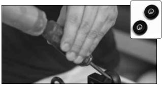
**6. NOTE:** If the rollers are not easily removed, gently tap the roller on inner metal ring of bearing as shown, with a flat head screwdriver and rubber mallet.
