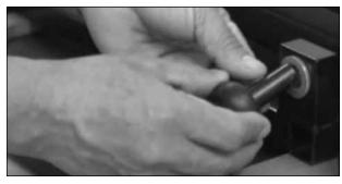
**2. To replace floating rollers.** Simply slide them out of the bronze bushings and carefully insert the new ones.
