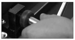
**3. To replace fixed rollers.** Use a ratchet tool and a 1/2" socket attachment.
