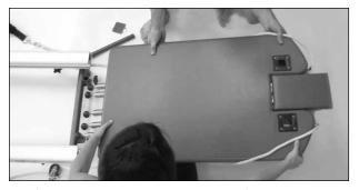
**7.** Before replacing carriage, wipe the inside of aluminum rails (c-channels) with a soft damp cloth. Find full instructions on page 23 of your Reformer Owner's Manual or view video online at merrithew.com/support/equipment-manuals-assembly
