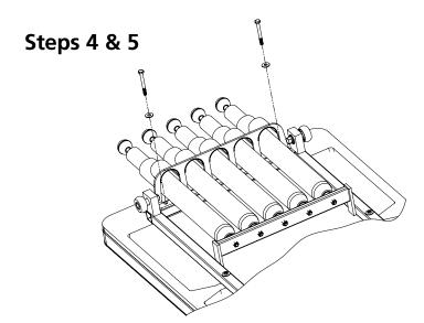
**4.** Place new washers over the metal spring holder bolt holes. Screw the bolts down through the holder and carriage frame until it is firmly secured using a 7/16" (11.1125 mm) wrench.
