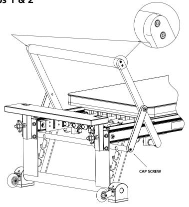
After frequent use, the fasteners for the footbar mechanism may loosen and as a result, the footbar may angle upwards slightly at one end.
