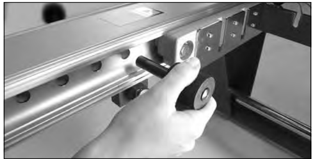
4. Adjust carriage stopper to position #1 (closest to wooden standing platform).
