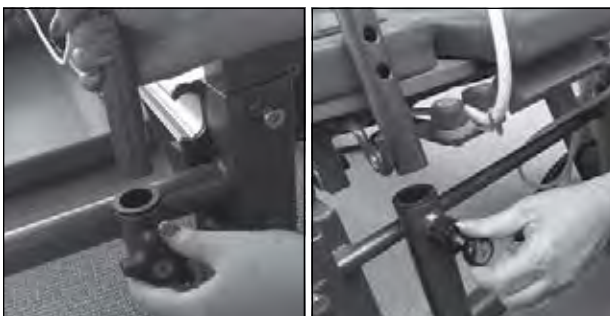
5. SPX MAX: Insert pulley posts [27] into receptacles [23] at back of Reformer and tighten star knobs [36]. Ensure eyehooks [52] on top of pulley posts are parallel to rails.
