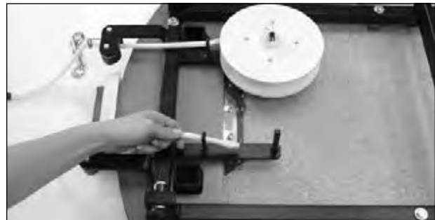
6. Feed straight end of new rope through eyehook projecting from reel bracket. This is the end of the rope to use in step 7.
