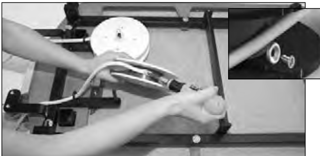
5. Undo screw and separate from rope [24]. Retain screw and cup washer. Remove old rope and discard.
