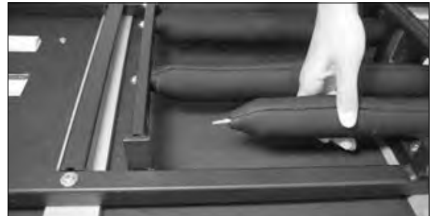
4. Remove spring bolt [31] from spring anchoring bar [40], then pull ball end of the spring out of holder [33].
