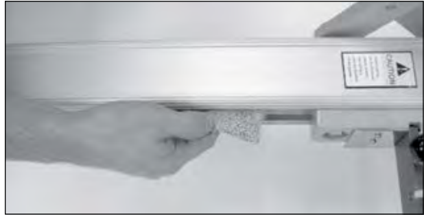
2. Wipe inside of aluminum rails (c-channels) [51] with a damp cloth using water only to remove dust or dirt. Spray onto cloth first. Avoid spraying liquid directly onto surfaces, rollers or rails. Insert carriage stopper [47] in one of six positions.
