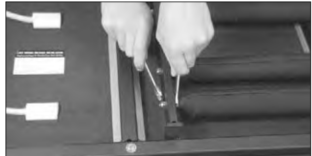
2. With two 7/16" wrenches or pliers, hold fixed cube nut [30] in place.
