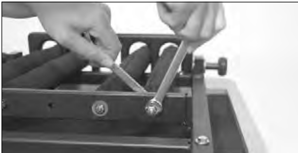
3. Using second 7/16" wrench on opposite side of spring anchoring bar, loosen nylon locknut [32]. This may require exerting a bit of torque.
