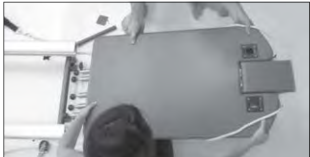
4. Align fixed rollers [37] with c-channels [51], then adjust floating rollers [38] as necessary before guiding carriage [15] into rails [14].
