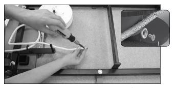
**7.** Place screw and cup washer directly in the center of replacement rope, 1/2" from the end and thread completely through rope.
