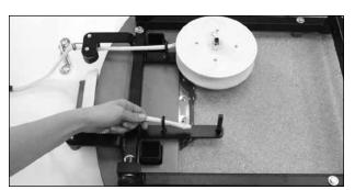
**6.** Feed straight end of new rope through eyehook projecting from reel bracket. This is the end of the rope to use in step 7.
