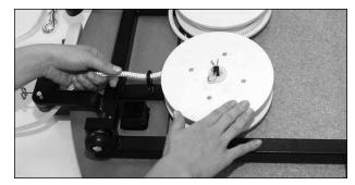
**11.** Wind rope around rope housing reel so rope lays flat against hub. There should be some resistance on reel and you should hear clicking as spring mechanism engages. Recoil full length of rope.
