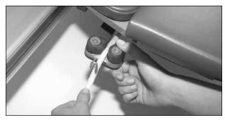
**12.** Before replacing carriage, wipe rollers and inside of aluminum rails (c-channels) with a soft damp cloth. *Find full instructions on page 23 of the Reformer Owner's Manual or view video online at* **merrithew.com/support/equipment-manuals-assembly**
