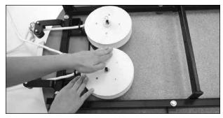
**8.** To determine the direction rope must coil, place empty reel on square shaft. Rotate reel in each direction. An audible clicking sound will indicate the correct direction to wind reel.
