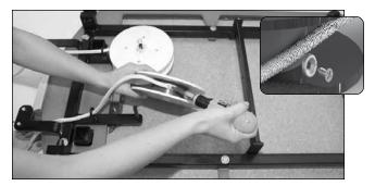
**5.** Undo screw and separate from rope. Retain screw and cup washer. Discard the old rope.
