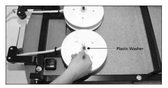
**3.** Pull out cotter pin and remove plastic washer from rope housing reel.
