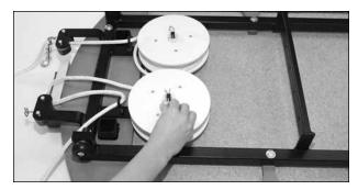
**10.** Place reel back on square shaft and replace plastic washer. Secure cotter pin so middle curve fits over square shaft.
