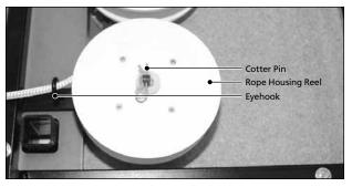
2. Locate rope housing reels on the underside of the carriage.
