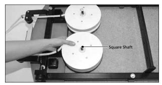
**4.** Remove rope housing reel from square shaft and uncoil rope.
