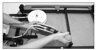
**9.** Remove reel. Place screw in the pre-drilled hole located on the grey plastic hub of reel and affix rope securely. Screw in completely without over-tightening.
