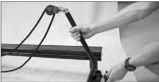
7. Insert pulleybars into receptacles at rear of Reformer and fully tighten star knobs so pulleybars are secure. Ensure eyehooks on top of pulleybars are parallel to aluminum rails.
