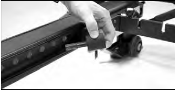
1. Remove carriage stopper.
