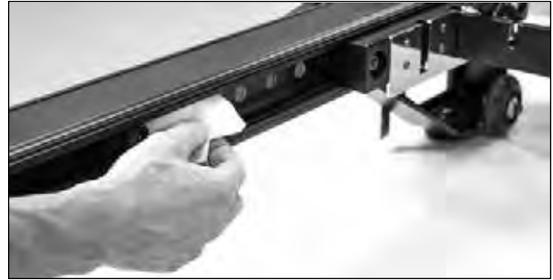
2. Wipe inside of aluminum rails with a dry cloth to remove dust or dirt. If using a damp cloth, spray cleaner onto cloth first. Avoid spraying directly onto surfaces, rollers or aluminum rails. Insert carriage stopper in one of six positions.
